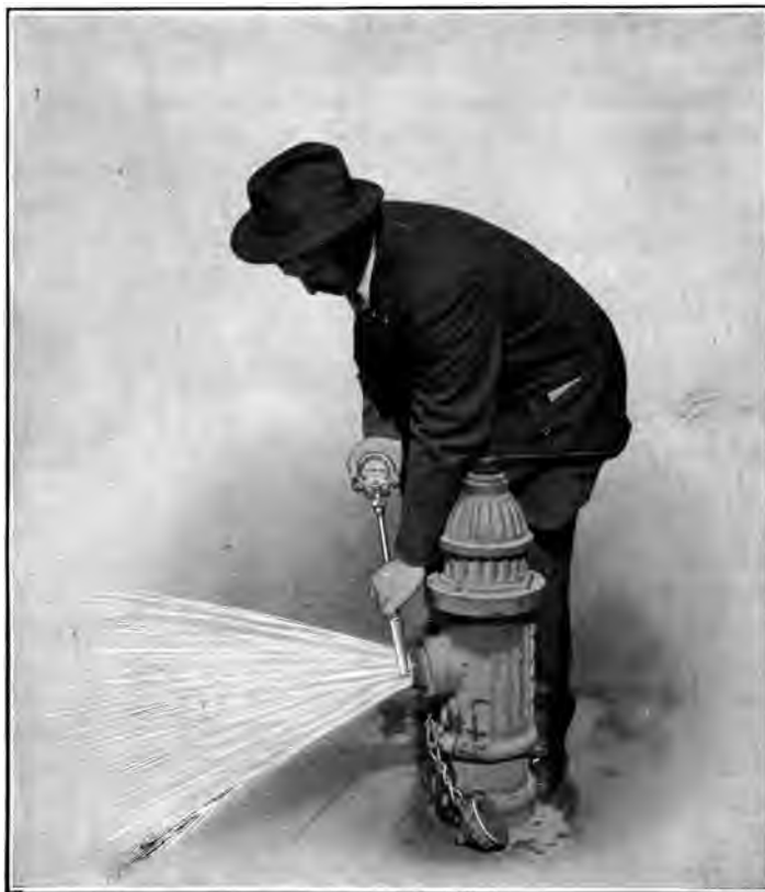
FIG. 229a. — Gauging Flow of Hydrant with Pitot Tube.
